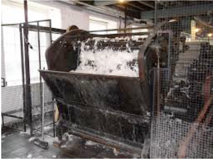
Picture of hopper where the blended wool was placed at the start of the blending process
